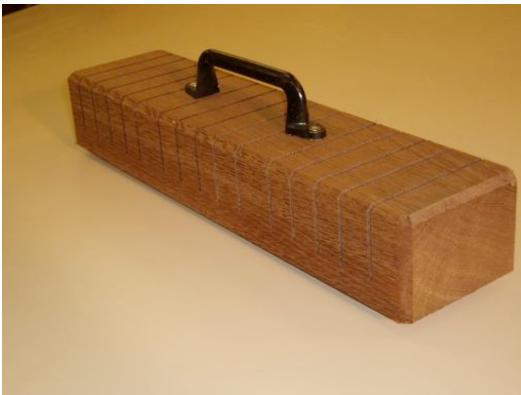
Proposed Sacrificial Lure Trap for Anobiid eggs
